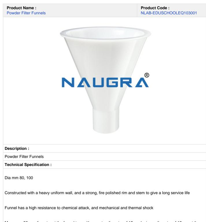
Measures 80mm diameter at the funnel top, with an outer diameter of 15mm by inner diameter of 12mm at the stem
